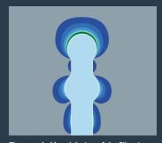
The rounded head design of the Fiber Lux and Fiber White reduce stresses in the core material and thereby prevent micro-fractures
