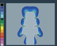
Posts that have heads with sharp edges or angles create stress points in the core material that can lead to micro-fractures
